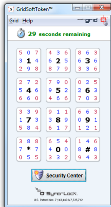
Figure 1: The user is presented with SyferLock GridSoftToken when requesting authentication. The password, or in this case PIN, is not presented to the user in the clear. Only the authorized user can input the PIN using SyferLock.
